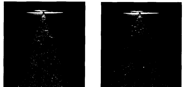
(a) Large Backhole (b) No Backhole Oxidizer Sprays of Swirl Coaxial Injector (Recess = 0)
