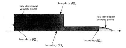
$\partial \Omega_1$ : essential boundary condition for velocity (v = 0)
