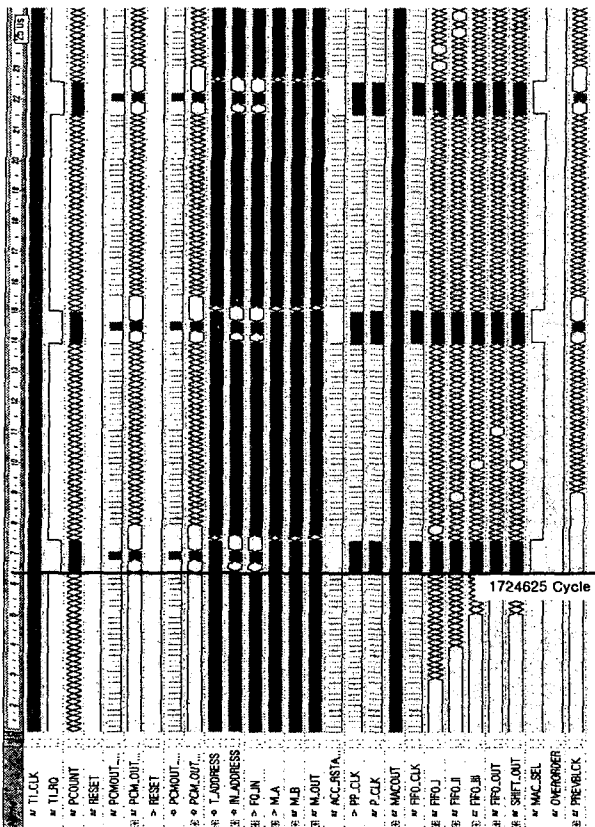
Fig. 10. The final PCM output of AAC decoding by DSP core proposed.
