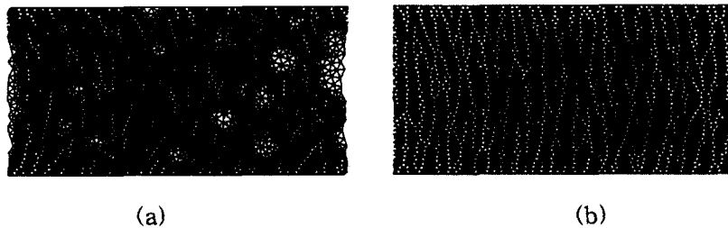
Fig. 2 Snapshots of particles in an ER fluid when electric field and pressure gradient are applied. (a) 10% volume fraction, (b) 30% volume fraction.
