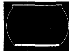
20 Mils Ball Diameter = 0.56 mm Height = 0.375 mm
