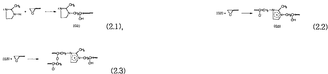
Figure 1. Simplified reaction mechanism for DGEFBF cured with Nadic methyl anhydride and 2MI.
