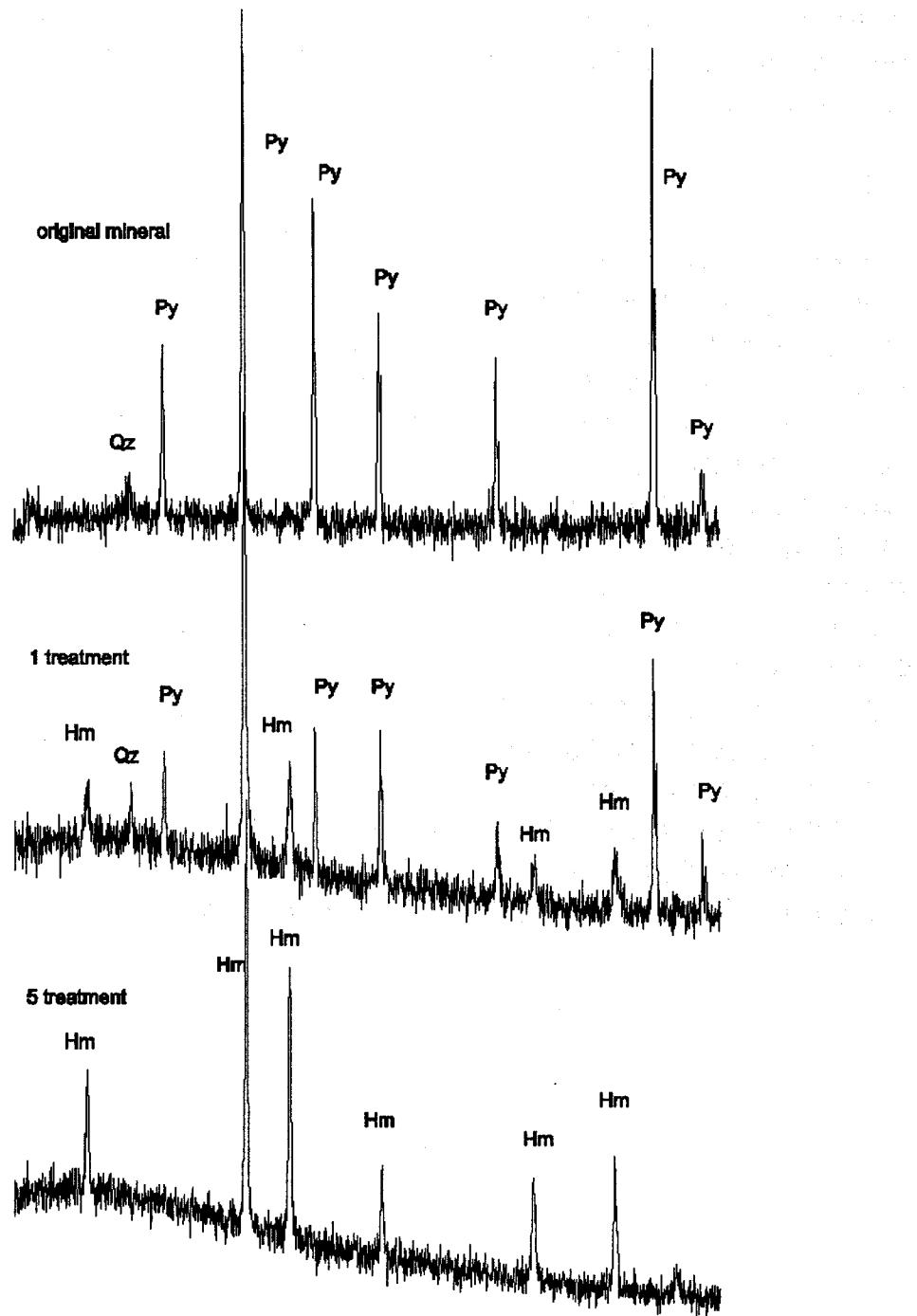
Fig. 1. XRD patterns representing mineralogical changes of pyrite after first and fifth refining treatments undergoing on 450°C-4hours heating and quenching.
