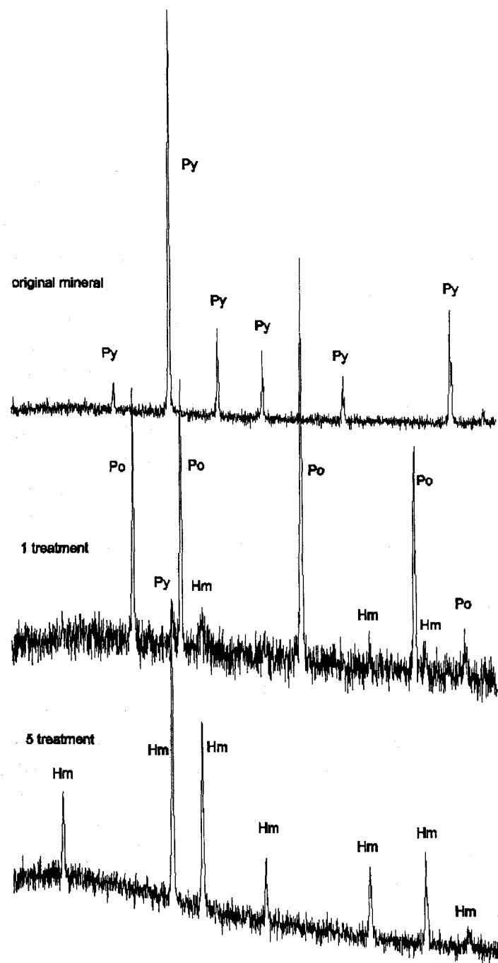
Fig. 2. XRD patterns representing mineralogical changes of pyrite after first and fifth refining treatments undergoing on 650°C-1.5hours heating and quenching.
