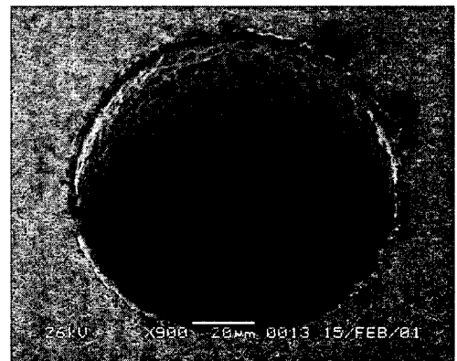
Fig. 6 Micro punching die made by MEDM (WC, \Phi 110 \mu\text{m} )
