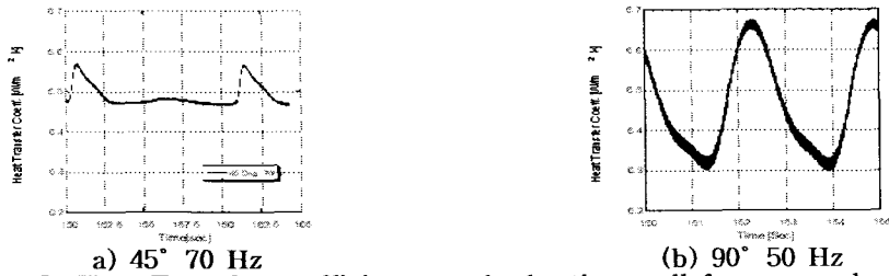
Fig. 8 Heat Transfer coefficients at the heating wall for one cycle
