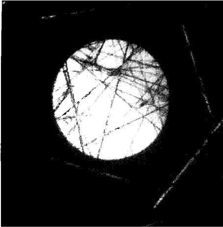
Fig. 2. HOLZ line of Albite [103] direction. TEM and exposure condition of 120keV, 37 \mu\text{m} C3 aperture size, 25nm spot size, and 5sec exposure time.
