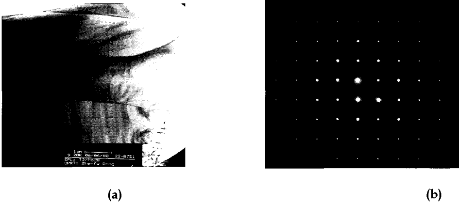
Fig. 5. (a) TEM image of the T 2 phase revealing a columnar growth and the growth direction and (b) electron diffraction pattern of the T 2 phase (001)
