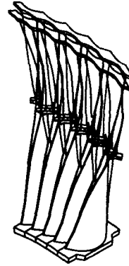
Fig. 11 The fundamental group axial mode shape of 5-blade group
