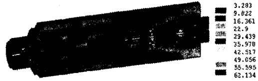
Fig. 4 Temperature distribution of spindle system (spindle speed : 30,000rpm)
