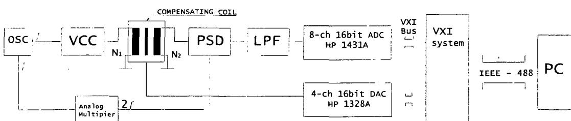
Fig.1 Schematic diagram of the constructed self compensating type flux-gate magnetometer
