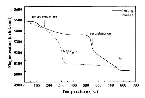
Fig. 1. TMA tracing of the Nd-Fe-B alloy high-energy ball milled for 48 hrs.
