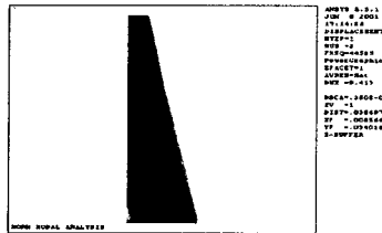
Fig. 3. Modal analysis of conical horn
