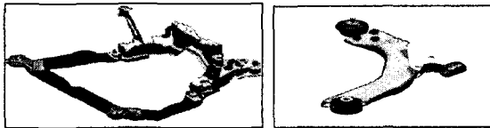
(a) Subframe (b) Lower arm Fig. 1 Hydroforming Designed 3D Model
