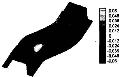
Fig. 8 Thickness strain distribution of S-Rail calculated by one step inverse analysis
