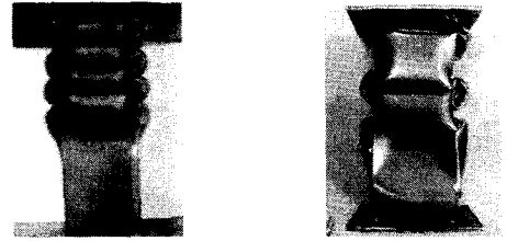
(a) A type specimen ( t/b = 0.055 )
