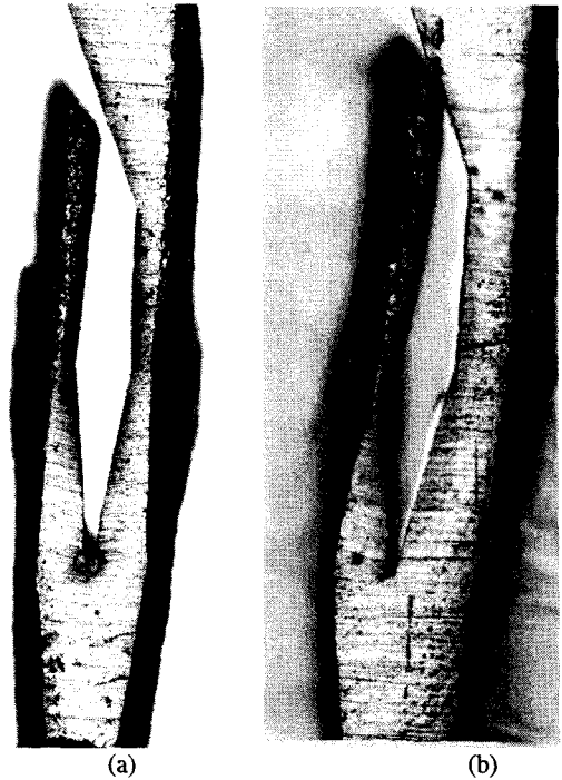
Fig.3 Deformed compliant press-fit pin
