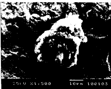
(b) Crack origin, H1SS, N_f=1.39 \times 10^6 cycles
