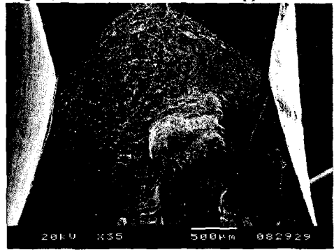
Fig. 7(f) Fracture Surface of 200 ppm H at 300°C
