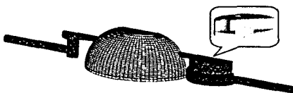
Fig. 4 Computational mesh for flow analysis
