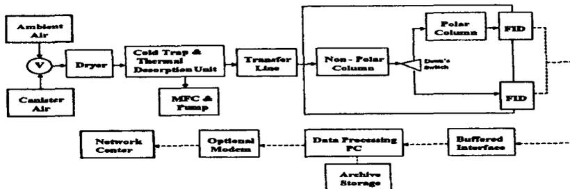
Fig. 1. Block diagram of the "On-Line System" for automatic monitoring of VOCs
