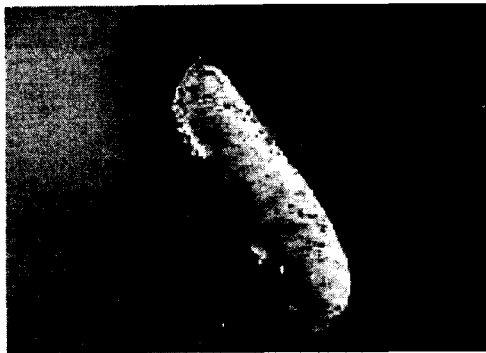
Fig.6 Crater wear observed from flank plane
