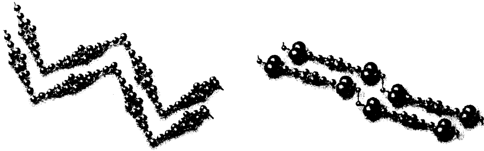
Figure 1. Chain conformation of PTT(a) and PET(b) polymers.[5]
