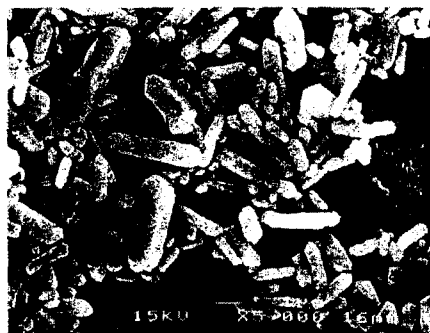
Fig. 1. Morphology of synthesized \alpha -SiAlON seed crystals.
