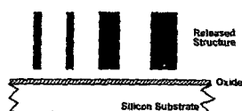
Fig. 4 Finally, the PMMA is removed. If desired, the customer can release the structures from the substrate by etching away the plating base in an \text{NH}_4\text{O}_2/\text{H}_2\text{O}_2 solution.
