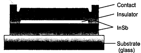
Fig.2 InSb Hall devices on the glass
