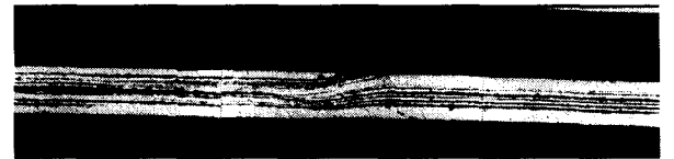
Figure 7. Optical micrograph of longitudinal cross section of jointed tape(right side)
