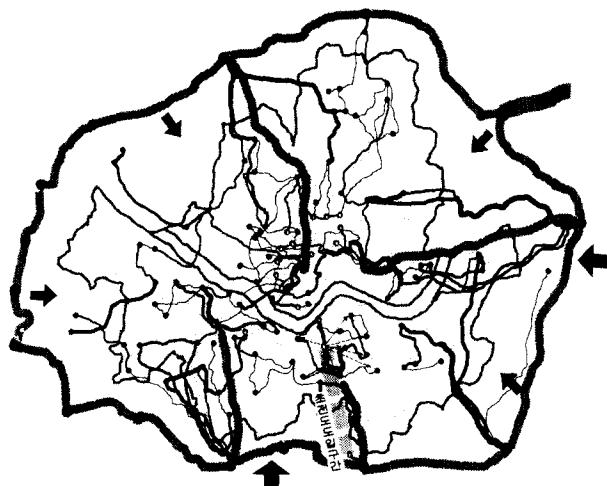
Fig 6. Power transmission system in 2035(application of the HTS power cable between metropolis and the middle area)
