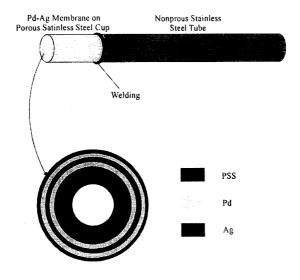
Fig. 1 Structure of a multiple layer Pd-Ag membrane
