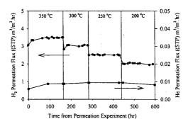
Fig.4 He and H<sub>2</sub> permeation flux through the Pd-Ag alloy membrane
