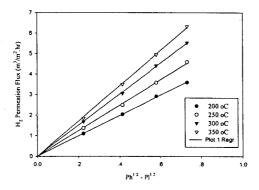
Fig. 5 Pressure dependency of H<sub>2</sub> permeation flux
