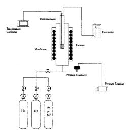
Fig. 3 Schematic diagram of gas permeation cell
