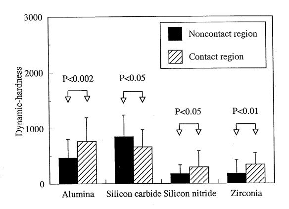
Fig.7 Dynamic hardness after wear test in bovine serum
