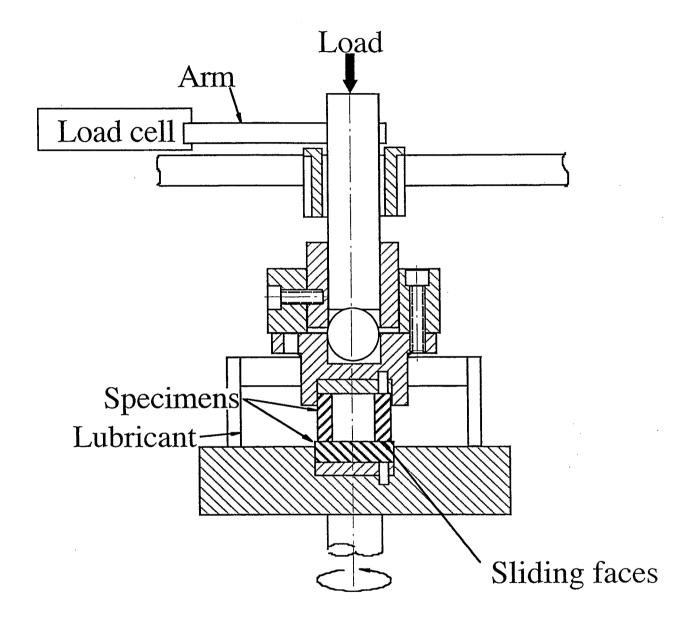
Fig.1 Schematic of end-face friction apparatus
