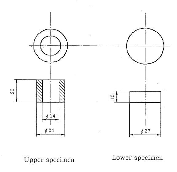
Fig.2 Shapes and dimensions of ceramic specimens
