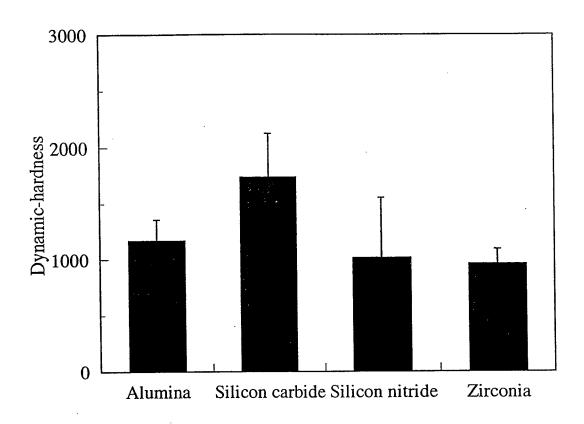
Fig.5 Dynamic hardness of original surface in micro scale
