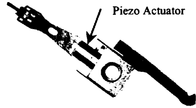
Fig. 2 Photography of a piezoelectric actuator
