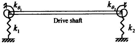
Fig. 4 System of drive shaft supported by joint element
