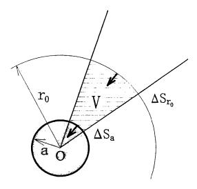
Fig.1. Schematic geometry of the proportinal counter. Here, a is the anode radius, and V represents the gas amplification region.  $\Delta S_a$  and  $\Delta S_{r0}$  denote segments of surface area for r=a and a=r<sub>0</sub>, respectively.  $\Delta S_a: \Delta S_{r0}=a^s: r_0^s$  (s=1 for cylindrical, s=2 for spherical).
