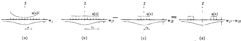
Fig. 3 The surface displacement due to a arbitrary axisymmetric loading
