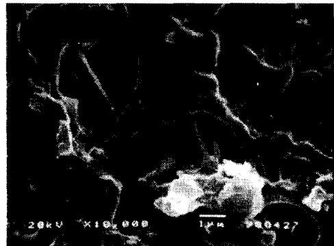
Fig. 5 SEM photomicrograph of notched Izod impact fractured surface of EPDM 32 tested at -30°C (fractured surface was treated with Xylene at 25°C for 10min).
