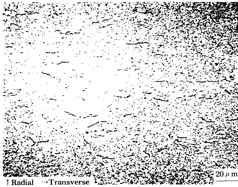
Fig. 3. Hydride Morphology of Radial Textured Tube.
