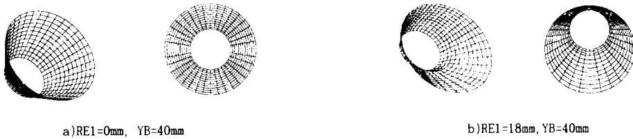
Fig. 3 The boundary surface of Dead Metal Zone
