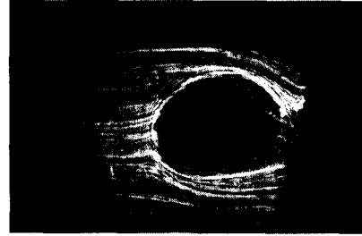
(d) K_{III} = 0.1931 [MPa·mm 3/2 ], Y_{max} = 31.6 mm Z_c = 30 mm, Z_0 = 662 mm, \lambda = 23.0666 (in case of inside axial directional crack)
