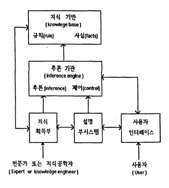
Fig. 1. Architecture of rule based expert system.
