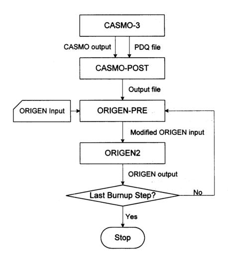
Figure 1. Data Flow Diagram for the CASMO/ORIGEN Coupling Program
