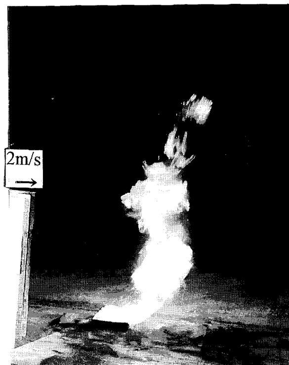
Figure 8 Typical swirling flame in a shear wind blowing through a vertical slit.
