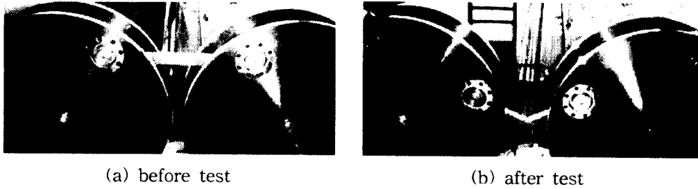
Fig. 4 Bending collapse test
