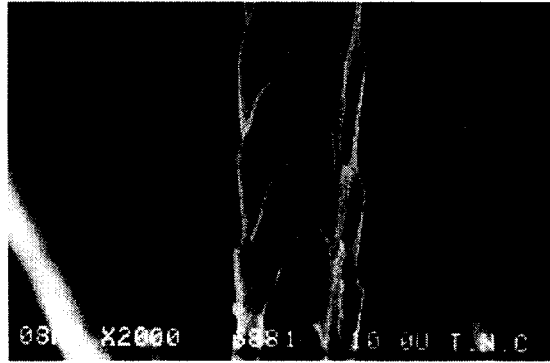
Figure 1. SEM photograph of no-moistured angora rabbit fiber treated with SO 2 gas for 30 seconds at 20°C.
