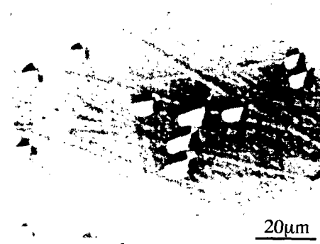
Fig. 6. Micrograph of the etched vicinal (0001)Si surface of a 6H-SiC [\bar{1}\bar{1}00] grown crystal.
