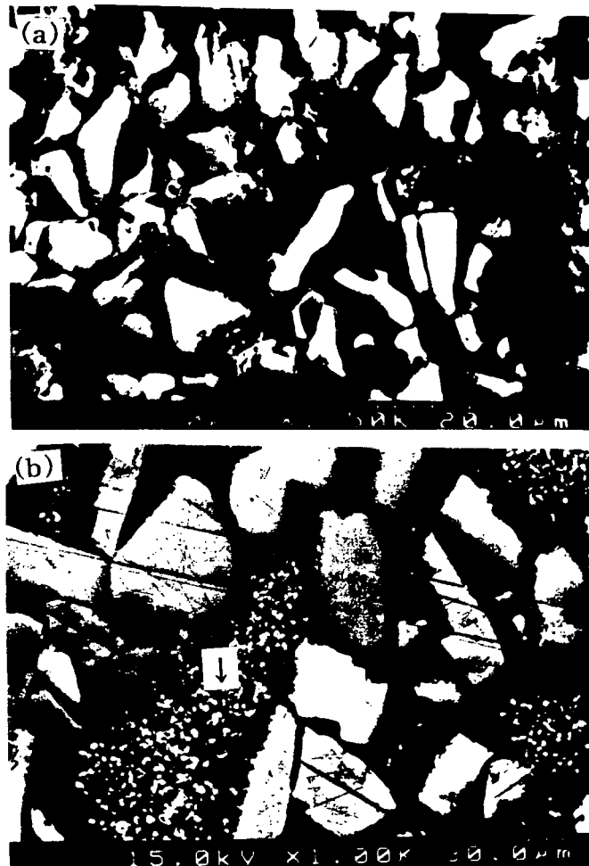
Fig.3. SEM microstructure of RBSC fabricated by a molten Si infiltration process ; (a)SG1 and (b)SG2
