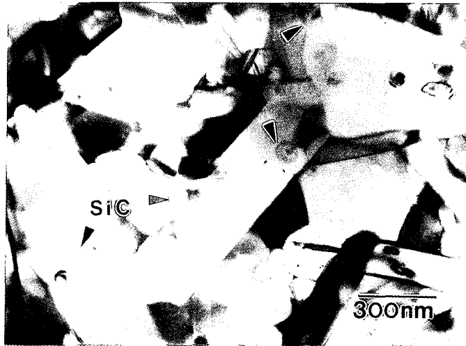
TEM micrograph showing that SiC particles are distributed both inside Si 3 N 4 grains and at grain boundaries.
