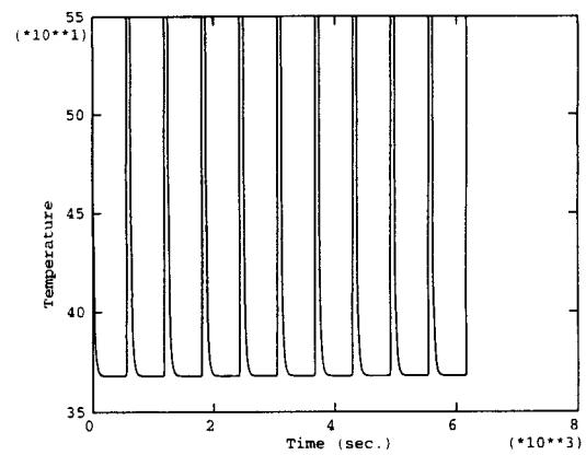
Fig. 2. Temperature history at bottom of the cylinder
