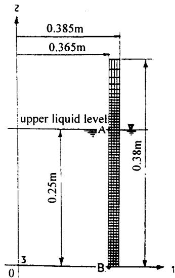
Fig. 1 Finite element model
